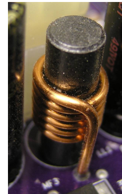
▲ An inductor is just a coil of wire. Its electrical properties derive from the magnetic field it creates when current flows through it.
